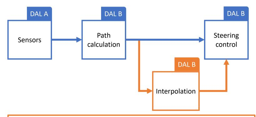
The decision of which function to keep running in case of a fault should not be based on criticality only
