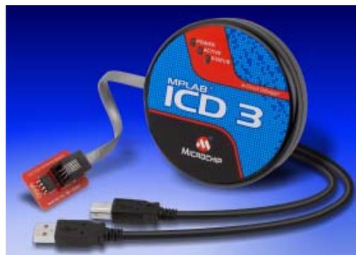
**Figure 3.2:** The MPLAB In-Circuit debugger [31]
