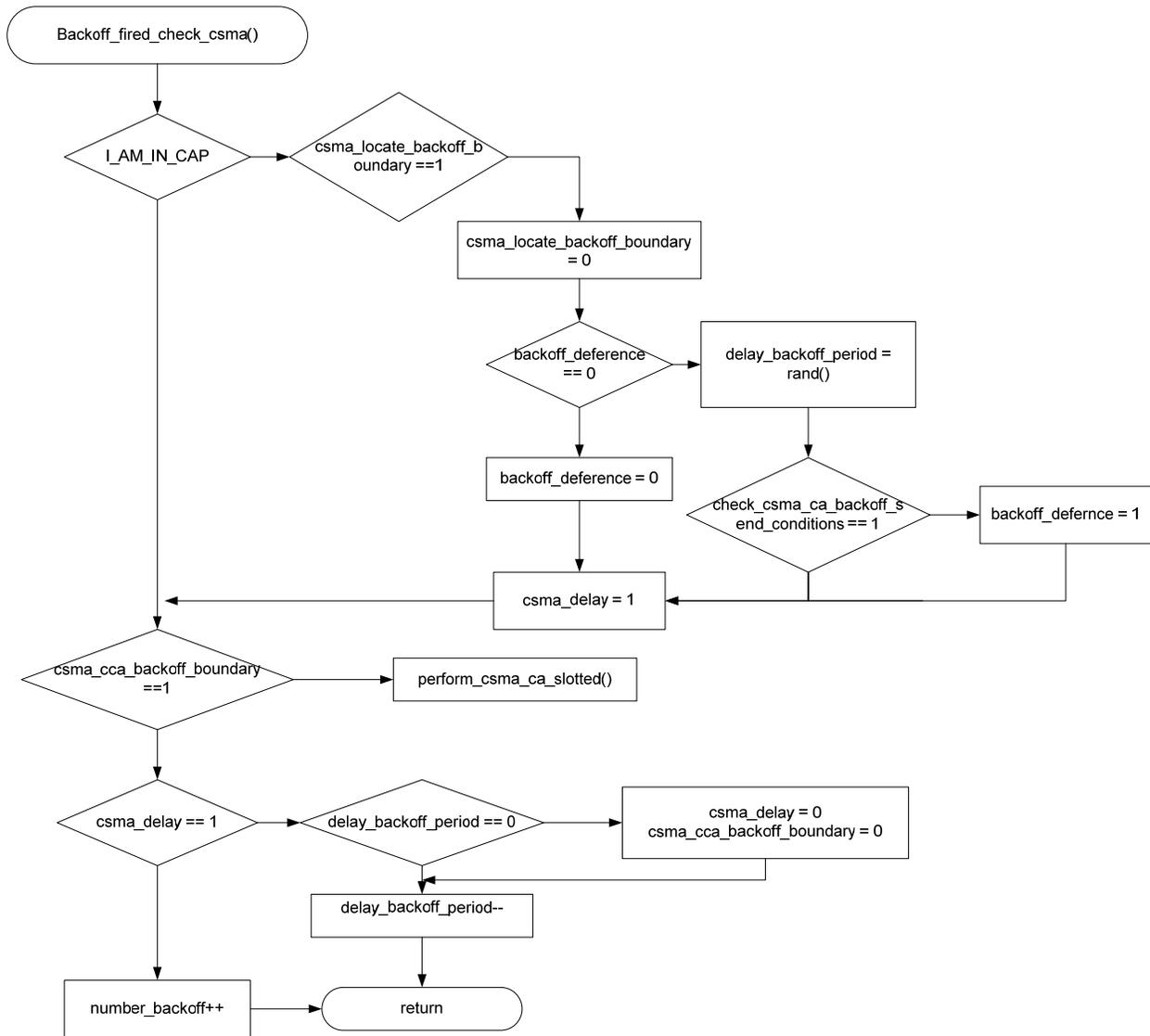
Figure 4.16: *backoff\_fired\_check\_csma\_ca()* function flowchart
