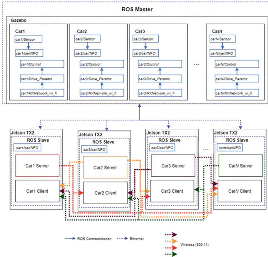
Fig. 5. System Architecture
